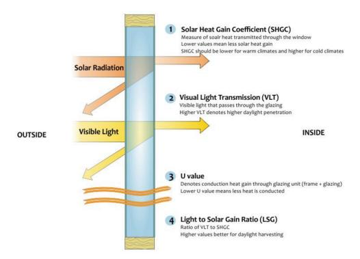
In conclusion, over the course of many decades, glass manufactures have been able to increase the number of active silver and dielectric layers in low-e coatings without increasing the thickness of the coatings. This has enabled them to make low-e architectural glass highly transparent while simultaneously increasing their ability to reflect heat energy.
