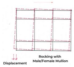
Rocking is common among unitized assemblies and allows the frame to rotate up while mostly maintaining its rectangular or square position. These frames require mating vertical and horizontal engagements as well as anti-walk blocks, and may still have some degree of racking.
