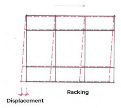
Racking is common among stick framing systems and results in the framing going diagonal, forming a parallelogram. The important issue in using this method of compliance is the utilization of anti-walk blocks and that there is adequate clearance of the glass to frame.
