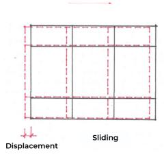
Sliding is again common in unitized assemblies where the frame is allowed to travel with the floor displacement, mostly maintaining its rectangular or square position. These also require the use of anti-walk blocks and will normally require more of the movement to be taken in the mating engagements or sealant joints.
