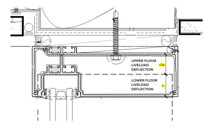
Live load deflection should also be designed into the other façade systems, such as nesting stud tracks in rainscreen applications. It is also common to find systems that span between columns, such as precast panels, which may not require the accommodation of center of beam deflection. Again, evaluation of all façade systems is necessary for a coordinated solution.
