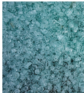
Broken pieces of toughened or tempered safety glass.
